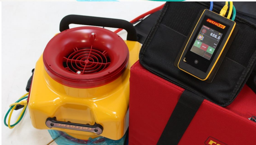
Retrotec DucTester completely sealed creates 656 Pa and flow reads correctly at 0 CFM.
