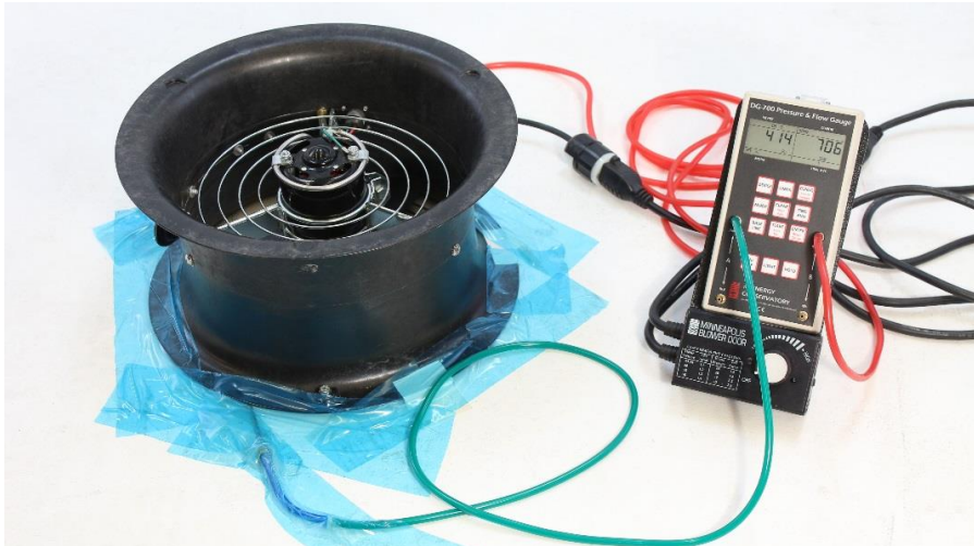
TEC Duct Blaster when completely sealed at the outlet creates 414 Pa and flow reads 706 CFM even though it's actually zero.
