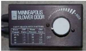
Triac circuit for speed control on power cord. Manual speed control attached to power cord.
