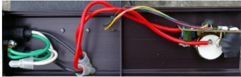
Triac circuit for speed control on power cord. Manual speed control attached to power cord.
