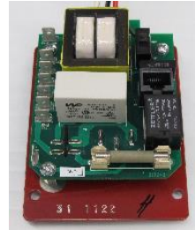
Regulated steady speed control inside fan produces better control with less overheating. Can be controlled over 100 meters using CAT 5 cable.
