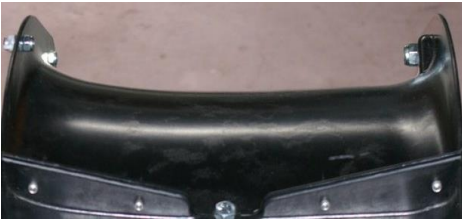
Fiber reinforced 2 piece injection molding held together with 4 rivets on flange
