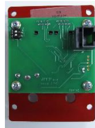
Regulated steady speed control inside fan produces better control with less overheating. Can be controlled over 100 meters using CAT 5 cable.
