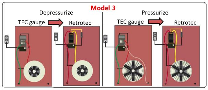
Figure 5: Comparison of connections using a Retrotec gauge instead of the TEC gauge using Model 3
