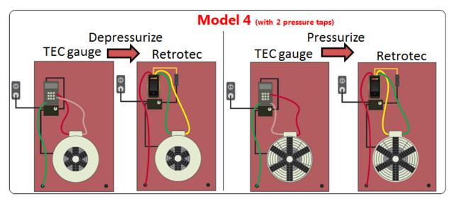
Figure 7: Comparison of connections using a Retrotec gauge instead of the TEC gauge using Model 4
