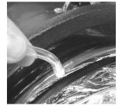
Figure 10: Duct Blaster Flow conditioner plastic tap\*
