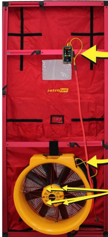
2-channel gauge that provides a reading for both pressure and flow. The DM-32 gauge also serves as the controls for the fan by automatically turning it on once a desired pressure is set.
