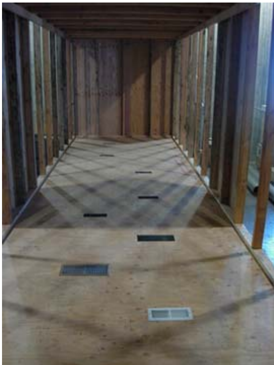
Figure A1. Photographs of test chamber construction showing registers located in the floor
