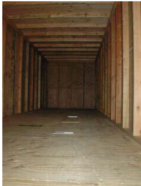
Figure A1. Photographs of test chamber construction showing registers located in the floor
