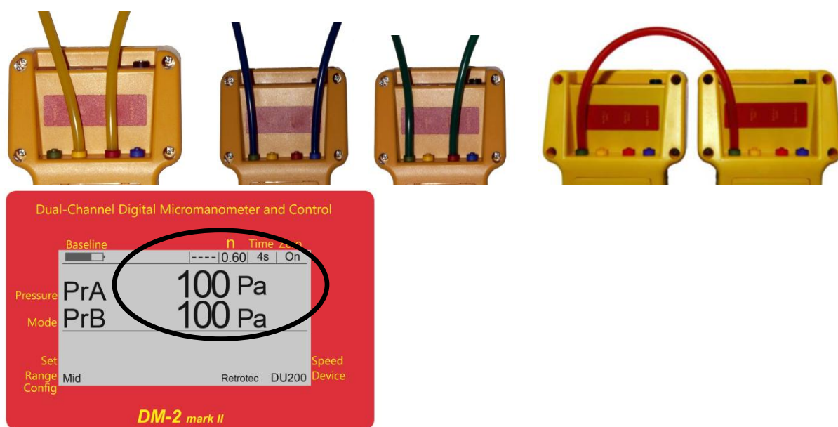
Figure 6: When a tube is connected between two ports and the readings on “PrA” and “PrB” are within 1%, the gauge is accurate.
