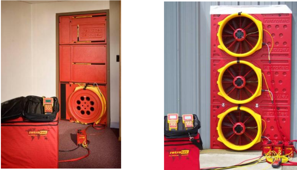
Fig.5.8 Fan-door System Installed in a Doorway with Single and Multiple Fans (Retrotec 2012)
