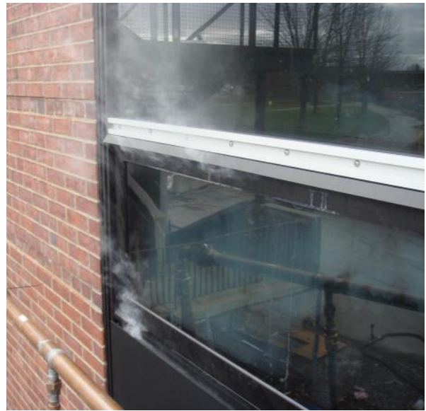
Fig.5.5 Diagnostic smoke testing of a window and window to wall interface while the suite is under positive pressure differential (Photo by Patenaude Trempe Inc.)
