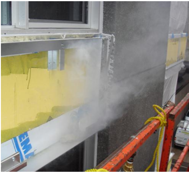
Fig.5.5 Diagnostic smoke testing of a window and window to wall interface while the suite is under positive pressure differential (Photo by Patenaude Trempe Inc.)
