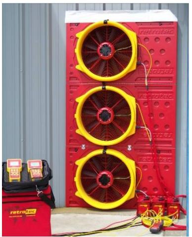
Retrotec Model QMG consists of one DM-2A, one DM-2, three 3300 Fans and a Light weight hard door panel for 3 fans. Add fan cases, software, grill mask and accessory options.
