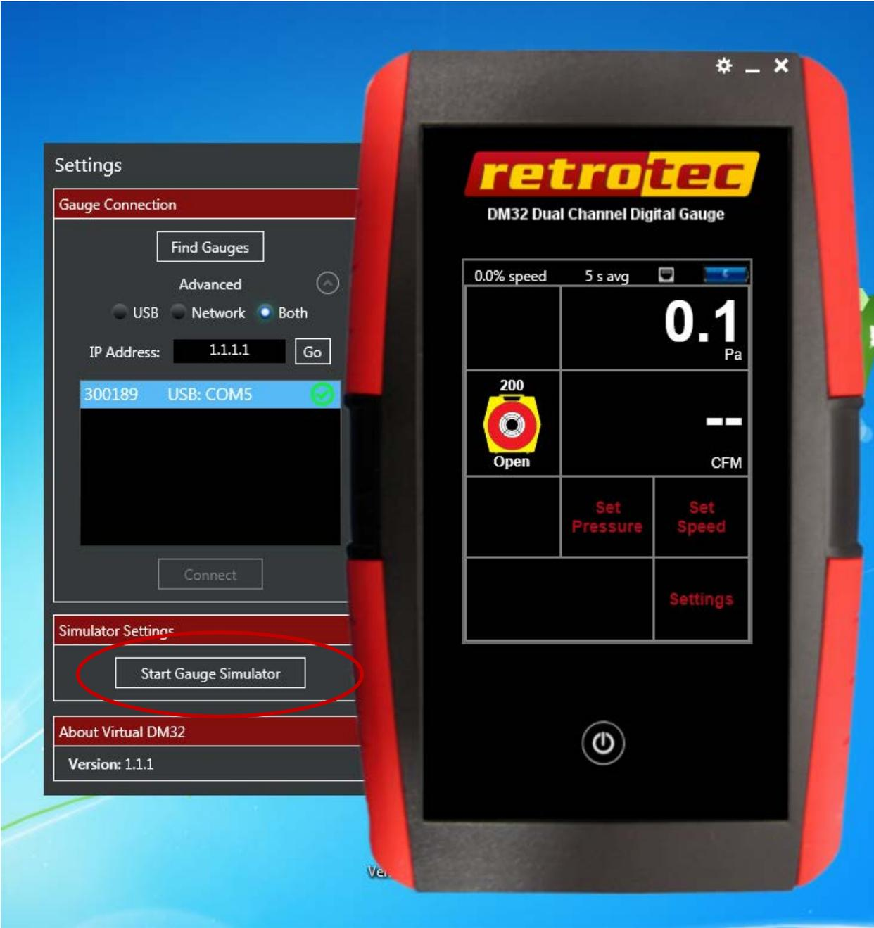
Figure 16: Click on [Start Gauge Simulator] to start a simulated gauge
