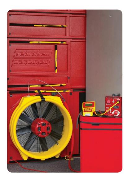
Controlling the flow of air through the exterior building enclosure is critical to reduce heat loss and heat gain and to minimize moisture-related problems. But controlling the flow of air between suites and common spaces within the building is also important. Anyone who has ever lived in an apartment building knows the unpleasantness of involuntarily smelling what the neighbor two floors below is cooking for dinner or smoking after dinner, and of hearing all about the neighbors' marriage
