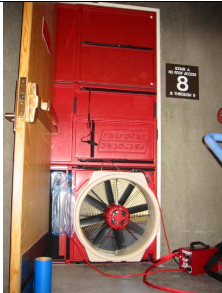
Rapid deployment panel sets up in seconds. Fan turns around to measure in the opposite direction.
