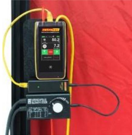
Figure 2: Attach Adapter inline between gauge Speed Control Output and Minneapolis Fan Speed Control Cruise Input
