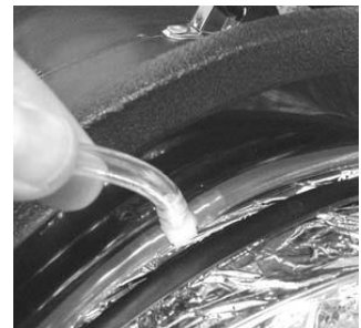
Figure 10: Duct Blaster Flow conditioner plastic tap*
