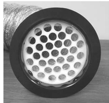
Figure 9: Flow conditioner installed for Depressurize\*
