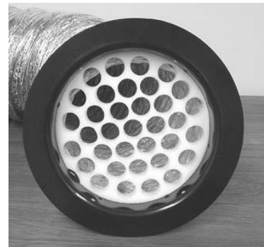
Figure 9: Flow conditioner installed for Depressurize*
