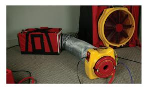
☐ To simulate a Duct Leakage to the Outdoors test, attach the Duct Leakage Simulator to one side of the tent. Open the slider between the house and duct simulator to create the leakage to the outdoors.
