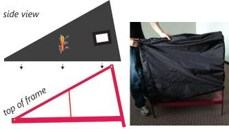
The bottom crossbar will be found attached to the frame inside of the cloth tent. Fold out and attach the bottom cross-brace to the base of the frame.
