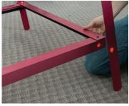
**Note:** the nylon washers are not required here as it is a non-moving part.
