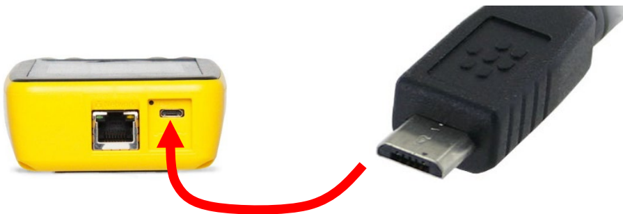
Figure 13A: Electrical connections on the bottom of the DM32 include Network (Ethernet) Cable that goes from the DM32 to a PC (if Retrotec PC software is used for data collection), micro USB cable for PC software and/or charging, and a reset
