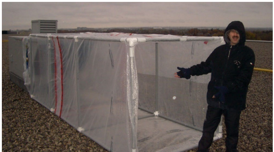
Figure 41 Tent made of poly and PVC pipe courtesy of Terry Brennan of Camroden Associates
