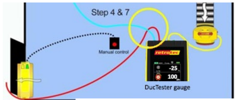
Figure 31: 1 Gauge Duct Leakage to Outdoors under depressurization, setting the duct pressure
