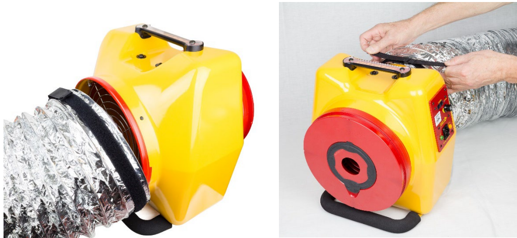
Figure 22: Install Flex Duct over the fan exhaust, for pressurization. Tighten the strap.
