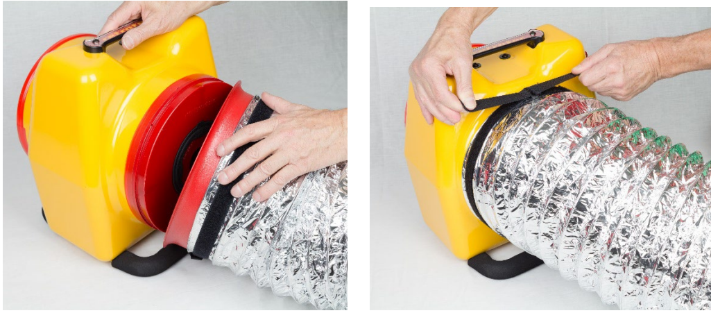
Figure 21: Install Flex Duct over the fan inlet, covering the Range Rings, for depressurization. Tighten the strap.
