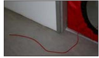
Note: Water in the tube will result in erroneous readings.
