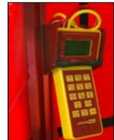
Place gauge case near fan, or attach gauge to Door Panel.
