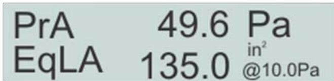
Note: Equivalent Leakage Area (EqLA) describes the leakage area in terms of one large hole in a flat surface. Unlike flow, EqLA is fairly consistent at different test pressures, but is usually referenced to 10Pa.
