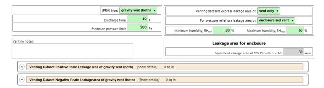
When any of the PRV types that provide venting only in the positive direction are chosen, only the positive venting dataset is used, and leakage area for negative pressure relief is assumed to be the "Total Enclosure Leakage".
