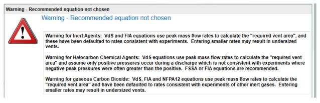
If you choose to use equations relying on peak mass flow rate to calculate peak pressure and minimum leakage required to relieve the peak pressure, entering smaller peak flow rates to override default values may result in under-estimating minimum venting area required. Such an under-estimation would lead to over-pressurization if a smaller than necessary vent is installed.
