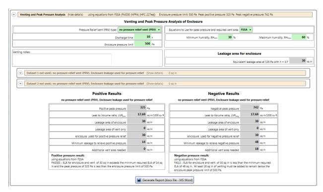
In the "Venting and Peak Pressure Analysis" section, there are 2 data sets that may be used to describe the venting area available during hold time, as well as the "Leakage area for enclosure" which was measured (or entered directly) in the "Hold time analysis- Total Enclosure Leakage" section and which is displayed here again for convenience, with its value extrapolated to 125 Pa.
