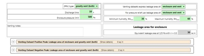
If the "Venting datasets express leakage area of:" drop down shows "vent only", datasets contain data which resulted from measuring or entering an estimate of the leakage area of the PRV itself. For measuring the positive venting dataset, the vents would have been fixed in the position they would assume under +125 Pa, and for the negative venting dataset, the vents would have been fixed in the position they would assume under -125 Pa.
