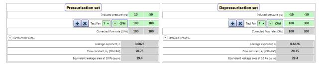
The reason behind performing an air leakage test in both directions is to average out any potential pressure problems there might be in one direction over the other (like blowing open a damper in one direction, but sucking it closed in the other).
