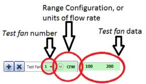
"Test Fan" data can be input as Fan Pressures, in units of Pa, (which allows FanTestic Integrity to calculate air flow rates through the Door Fan) or can be entered manually as air flow rates through the Door Fan, in units of CFM, m<sup>3</sup>/h, m<sup>3</sup>/s, or L/s.
