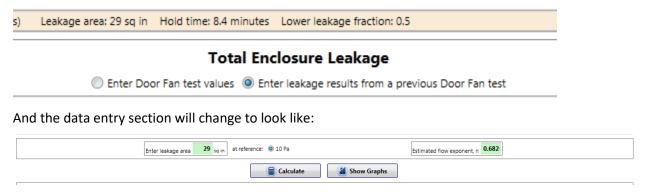
Enter the leakage area and the n value that was calculated in the previous Door Fan test.
