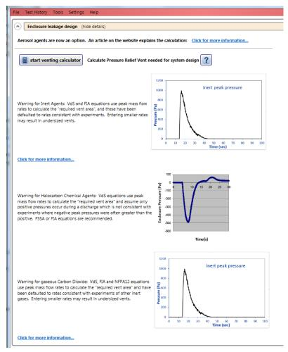
Alternatively you can click on the Tools menu and use the "Calculate Pressure Relief Vent needed for system design" menu option:
