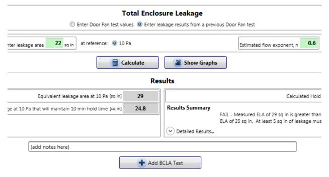
The test procedure for a BCLA test is the same as a Total Enclosure Leakage test, with the addition of some form of neutralizing the leaks that are occurring from the upper part of the enclosure. The BCLA procedure is required to negate the leakage above the enclosure's suspended ceiling by neutralizing the ceiling space (with a Flex Duct), or by physically covering the entire ceiling space (with sheets of plastic air barrier).
