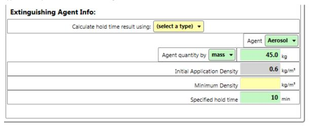
Choose "Continuous Mixing" as the method to use for calculating hold time. Enter the mass of agent as usual, and then FanTestic Integrity will calculate the "Initial Application Density" based on the volume of the enclosure you have entered. You then enter the "Minimum Density" allowed to extinguish the fire and the specified hold time.
