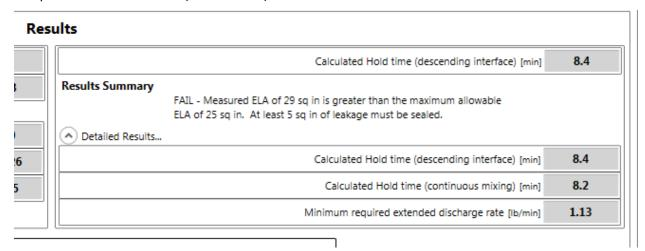
If your test has failed, you need to seal up enclosure leakages to lower the "Hold time" or required "Extended discharge rate", depending on what "Test type" it is.
