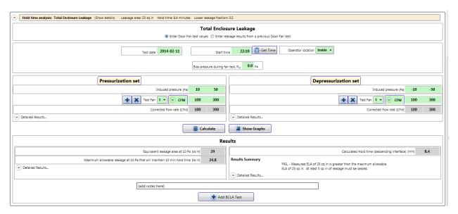
There are two methods to determine the total enclosure leakage – either enter recorded pressure/flow values from a door fan test performed on the enclosure and have FanTestic Integrity calculate the leakage ("Enter Door fan test values"), or enter a known value for the enclosure leakage ("Enter leakage results from a previous door fan test").
