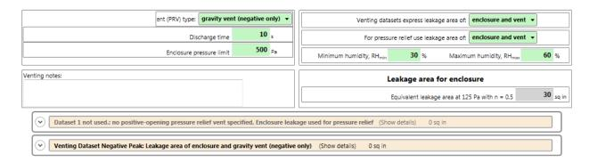
When any of the PRV types that provide the same venting area in both the positive and negative directions are chosen, only the positive venting dataset is used.
