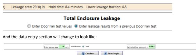
Enter the leakage area and the n value that was calculated in the previous Door Fan test.
