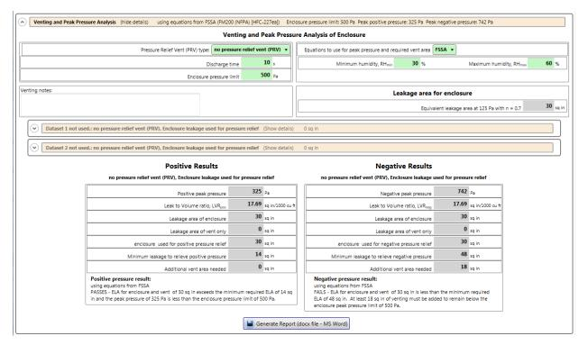
In the "Venting and Peak Pressure Analysis" section, there are 2 data sets that may be used to describe the venting area available during hold time, as well as the "Leakage area for enclosure" which was measured (or entered directly) in the "Hold time analysis- Total Enclosure Leakage" section and which is displayed here again for convenience, with its value extrapolated to 125 Pa.
