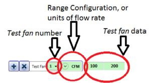
"Test Fan" data can be input as Fan Pressures, in units of Pa, (which allows FanTestic Integrity to calculate air flow rates through the Door Fan) or can be entered manually as air flow rates through the Door Fan, in units of CFM, m<sup>3</sup>/h, m<sup>3</sup>/s, or L/s.
