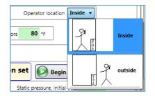
Select whether the operator is located inside or outside the enclosure during the test (inside is typical). Operator location is used in conjunction with the sign (positive or negative) from the "Induced pressure" readings, to determine the test direction (Pressurization or Depressurization).
