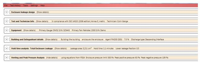
The expander will not be enabled and you will not be able to open it if the agent has been chosen as Aerosol. See the document "Explaining Aerosol Calculations" online for details, also accessible from within the program:
