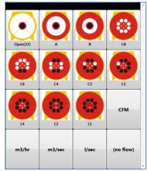
You can also enter the Fan Pressures by entering the "PrB" readings from the Retrotec gauge, along with the Fan Range configuration in use, so that FanTestic Integrity can calculate the Flow. When Fan Pressures are entered, you must select the Range
