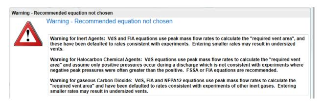
If you choose to use equations relying on peak mass flow rate to calculate peak pressure and minimum leakage required to relieve the peak pressure, entering smaller peak flow rates to override default values may result in under-estimating minimum venting area required. Such an under-estimation would lead to over-pressurization if a smaller than necessary vent is installed.
