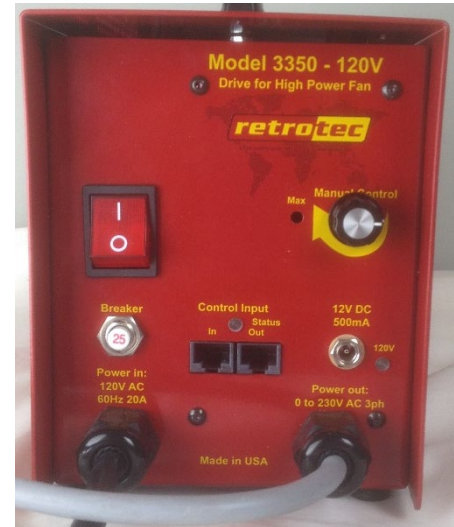
Figure 29: Cable ports on Model 3350 fan drives from 2012 and later.
