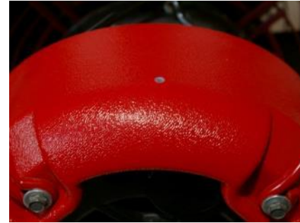
Figure 18: Pressure sensor on the fan motor casing.
