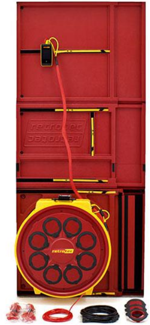
Figure 14: Modular door panel set installed.
