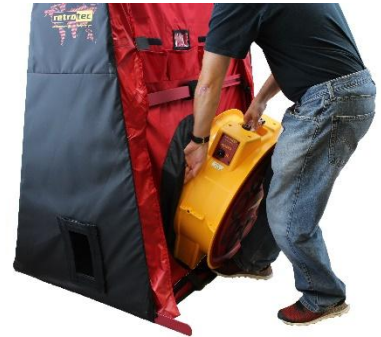
Figure 12: Installing a fan in the cloth door panel.
