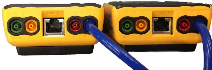
Gauge field check configuration: Cross gauge check
