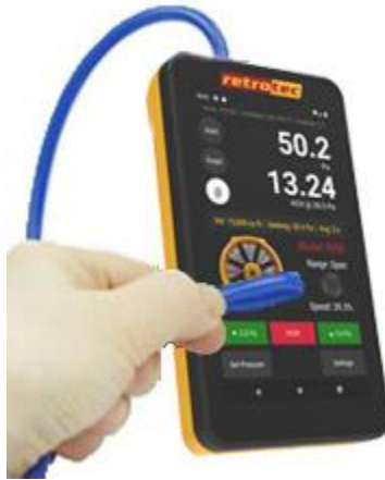
Errors in pressure reading from a pinched tube.
