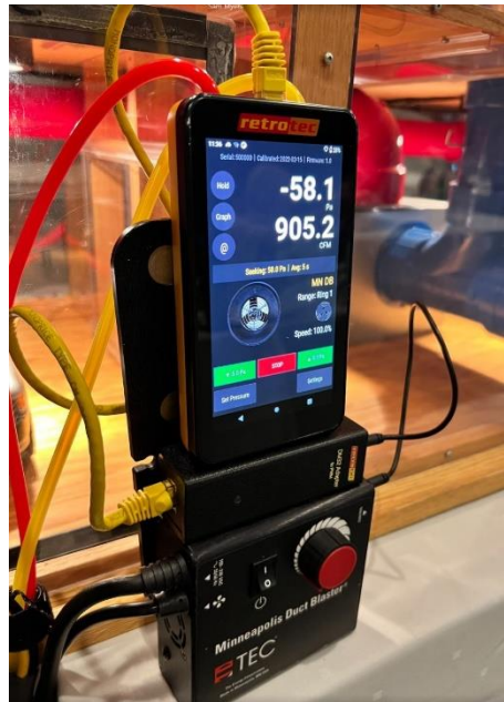
Control a TEC fan using the gauge and Fan Speed Control Adapter (part FN275, produced by Retrotec)
