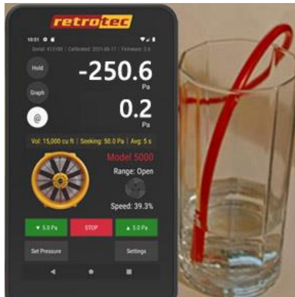
The gauge displaying a negative pressure (-250.6 Pa).
