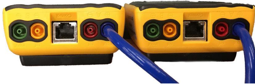
Gauge field check configuration: Cross gauge check
