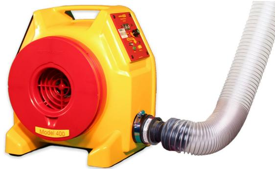
A Flow Conditioner is not needed with Retrotec fans for depressurization testing. Some duct testing fans require a flow conditioner when depressurizing a duct system, in order to get correct readings. The Retrotec DucTester does not require a flow conditioner because it uses a flow nozzle, which is intrinsically stable in either direction because the flow gets compressed as it goes through the nozzle.
