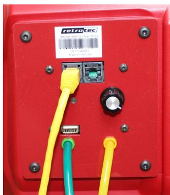
Figure 16: color-coded tubing connections (green and yellow) and Control Cable
