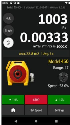
In the example on the left, the Device is set to “450” and Range to “47”. It is very important to ensure these are both correct. The Range is engraved in the orifice plate which also has a raised color sticker which is printed with “Range 47” in the case of this example.
