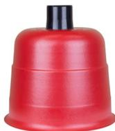
Adapters included have a 10 inch opening on one end that must fit over the inlet of the Test Blower for depressurization testing. The inlet end is 2.5 inches which accepts the 2.5 inch male connector on the flex.
