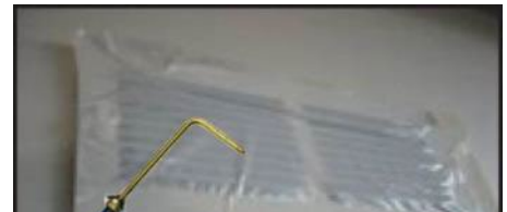
Figure 13: A Static Pressure Probe attached to a pressure tube allows the measurement of pressure without disturbances due to turbulence.
