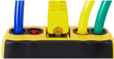
Figure 12: Pressure ports on the top of the gauge are color-coded to match the tubing
