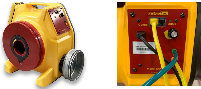
Figure 1: Retrotec Model 500 has a speed control knob and two Ethernet style Speed Control Ports for daisy chaining speed controls for running many fans together. The yellow and green color coded tubing connections to the gauge are shown.
