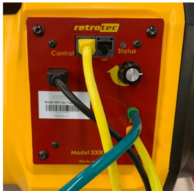
Figure 15: Model 500 Fan Top with power cord, color-coded tubing connections (green and yellow) and Control Cable.
