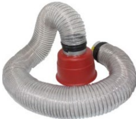
Figure 8: Flex Duct for duct testing system with 10 to 6 inch (254 to 152 mm) Adapter.
