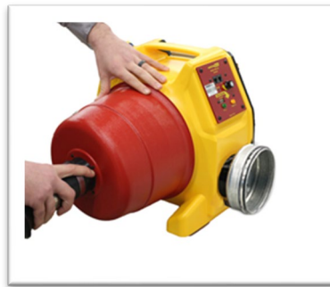
Figure 11: Install 10 to 6 inch Adapter over the fan inlet, covering the Range Rings, for depressurization.
