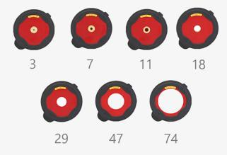
☐ Tap the image of the DucTester on the gauge and select the range to match your fan whenever a Range Plug is changed.
