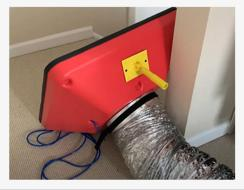
☐ Connect yellow and green tubes to matching color ports on the fan. Insert the blue tube into the blue port on the Powered Flow Hood.
