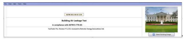
FanTestic is software designed to capture data and calculate results required for the analysis of building energy leakage based on one of a number of published Test Standards.
