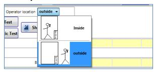
Select whether the operator is located inside or outside during the test (inside is typical). This is used in conjunction with the sign (positive or negative) from the Induced Pressure read from the gauge, to determine the test direction (Pressurization or Depressurization). The test direction will be displayed beside the Start time:
