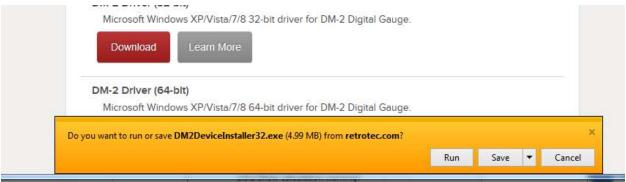
c) To install the Retrotec DM2 driver (DM2deviceinstaller32.exe or DM2DeviceInstaller64.exe), do not double click the file when the download has completed. Instead, right click the downloaded "DM2deviceinstaller" file, and select *Run as administrator* to start the installation. This will give permission to install the required system files.
