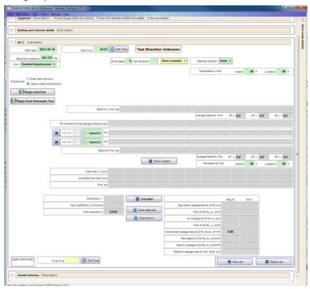
Data readings from each fan are specific to the range configuration installed on the fan when the pressure is read from the gauge. A Fan Pressure Line must be included in the set for each fan/range combination used during the test. New fan pressure lines must be added if ranges have to be changed during a test to reach the required induced pressure.
