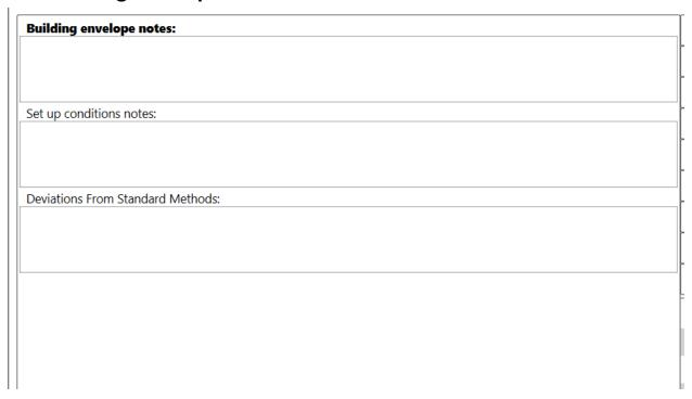
The tester can note any areas of major leakage in the building envelope, note the setup conditions for the test, and any deviations from standard methods.
