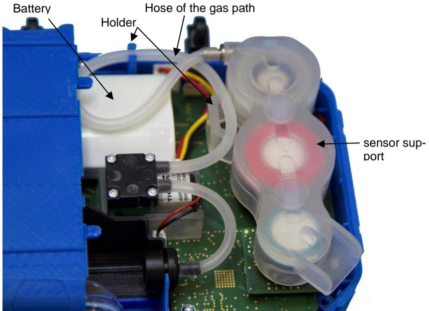
Fig. 49: Bottom of the analyzer with cover removed
