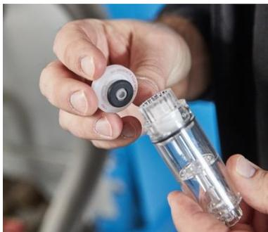
Fig. 46: Filter holder with water stop filter.
