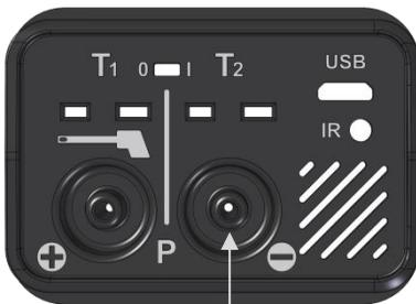
Fig. 27: Pressure connector
