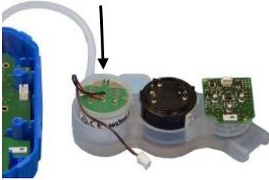
Fig. 51: Connector of the O<sub>2</sub>-sensor removed
