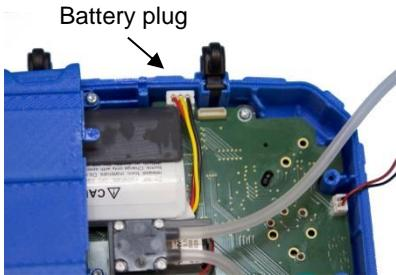
Fig. 55: Battery in the black adapter, sensors removed, O<sub>2</sub>-Sensor, plug and hose of the gas path are still connected.
