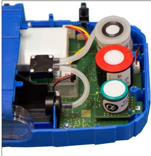
Fig. 52: Sensors plugged to the board. Top down: O<sub>2</sub>, CO and NO (option)
