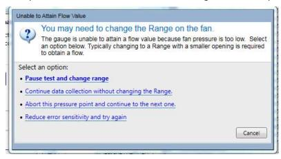
If you determine that you need to change the Range to complete the target point, click on "Pause test and change range", then physically change the range on the fan, and change the Range showing on the gauge. You will see the following in the Test Dashboard.
