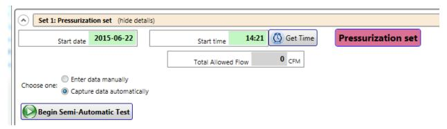
If the "Begin Semi-Automatic Test" button is not visible, click on the "Capture data automatically" choice. The software will ask if you want to lose any data entered.
