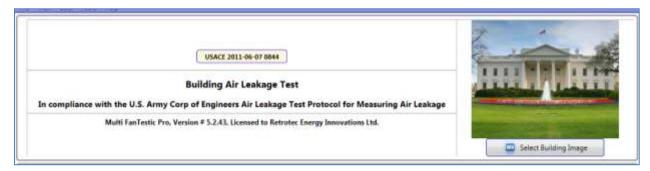
FanTestic is software designed to capture data and calculate results required for the analysis of building energy leakage based on one of a number of published Test Standards.
