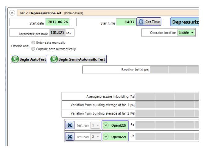
Data results can be added to the Set either manually or automatically.
