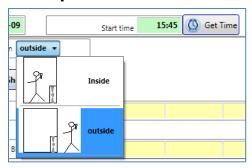
Select whether the operator is located inside or outside during the test (inside is typical). This is used in conjunction with the sign (positive or negative) from the Induced Pressure read from the gauge, to determine the test direction (Pressurization or Depressurization). The test direction will be displayed beside the Start time:
