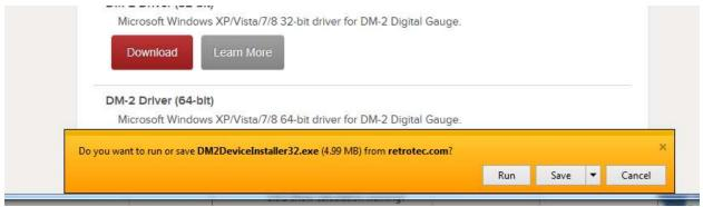
c) To install the Retrotec DM2 driver (DM2deviceinstaller32.exe or DM2DeviceInstaller64.exe), do not double click the file when the download has completed. Instead, right click the downloaded "DM2deviceinstaller" file, and select *Run as administrator* to start the installation. This will give permission to install the required system files.
