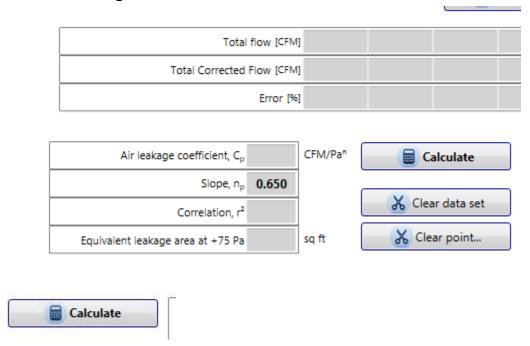
Click "Calculate" to force FanTestic to go through all the readings in the set and calculate the results.
