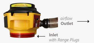
On Model 450 you can **depressurize** ducts by attaching the Adapter onto Fan inlet and attaching the Flex to it
