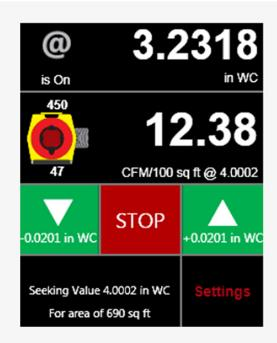
Connect Gauge to a laptop and have FanTestic run the test according to any Standard,
