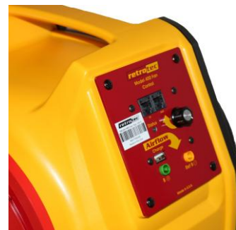
Figure 1: Retrotec Model 400 has a speed control knob and two Ethernet style Speed Control Ports for daisy chaining speed controls for running many fans together. The yellow and green color coded tubing connections to the gauge are shown.
