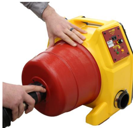
Figure 11: Install Flex Duct over the fan inlet, covering the Range Rings, for depressurization. Later systems have a 2.5 inch connector instead of the 4 inch (100 mm) shown.
