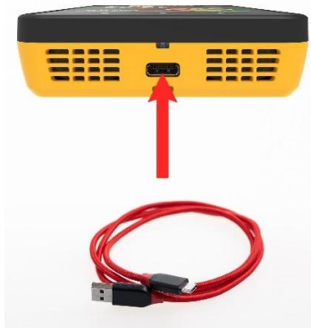
Figure 16B: The DM32X uses a USB-C Cable for charging, as well as for connecting to a PC.
