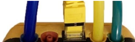
Figure 12: Pressure ports on the top of the gauge are color-coded to match the tubing.
