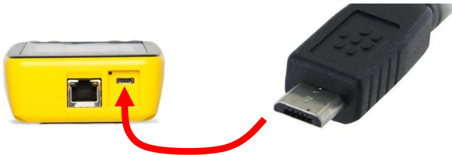
Figure 13A: Electrical connections on the bottom of the gauge include Network (Ethernet) Cable that goes from the DM32 to a PC (if Retrotec PC software is used for data collection), micro USB cable for PC software and/or charging, and a reset button. Flat portion of Micro USB must face down and rounded portion must face up for charging or connecting to your computer.
