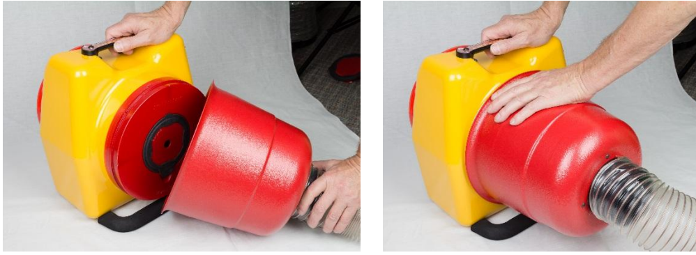
Figure 21: Install Flex Duct over the fan inlet, covering the Range Rings, for depressurization.
