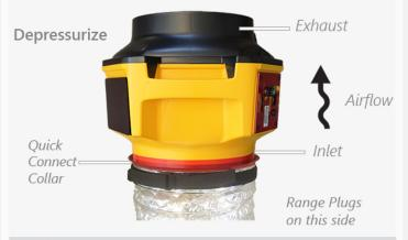
If Codes require you to pressurize, pass the test in the depressurize direction first then connect the Flex Duct to fan exhaust in order to pressurize. All other connections remain the same.
