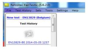
Make sure "New Test" on the history list is followed by "EN13829(Belgium)". If not, go to "Settings" → "Change Standard used for new tests" and change the test standard to "EN13829(Belgium)". You may need to restart the program if this change is not active immediately.
