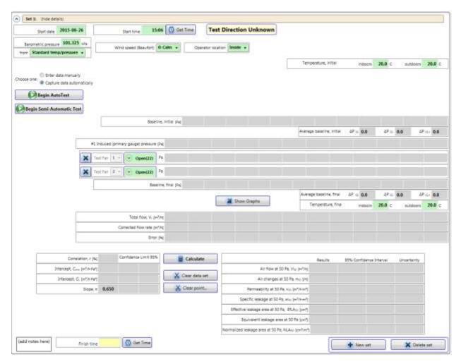
Data readings from each fan are specific to the range configuration installed on the fan when the pressure or flow is read from the gauge. A Fan Pressure Line must be included in the set for each fan/range combination used during the test (if ranges have to be changed during a test to reach the required induced pressure).
