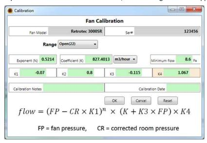
The equation displayed in the Fan Calibration window is the important thing to understand.
