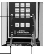
Connect the Green tubing to the Channel A Reference tap.
