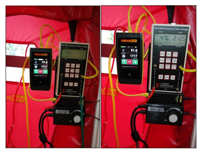
In this test scenario, both the outside reference tubing (red) and tubing reading the fan pressure (yellow) are split using nylon T connectors so that both gauges can take readings at the same time. A Retrotec speed control adapter is installed so that the DM32 has full control of the TEC fan. This adapter converts the TEC stereo jack to the Retrotec ethernet outlet.
