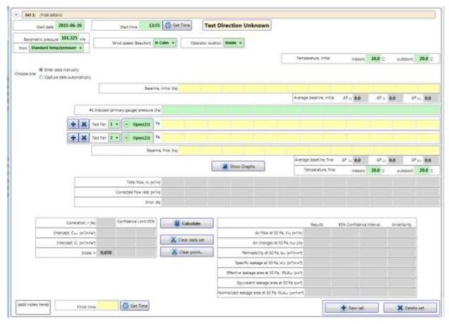
Data readings from each fan are specific to the range configuration installed on the fan when the pressure or flow is read from the gauge. A Fan Pressure Line must be added in the set for each
