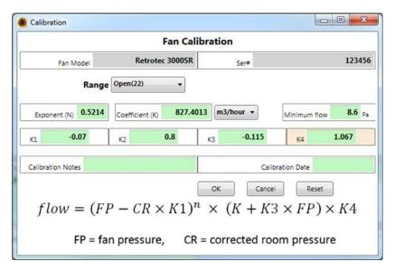
The equation displayed in the Fan Calibration window is the important thing to understand.
