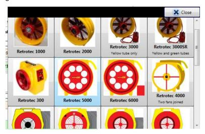
If you are performing a duct test, be sure to choose a Duct Testing fan, conveniently grouped together and shown in the picture with attached flex duct. Building test fans do not show the attached flex duct.
