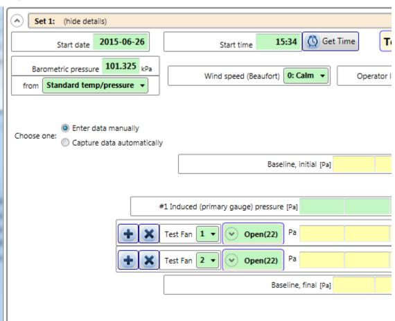
Each time you run another test after stopping for any reason, it is recommended that you add a new Set and delete the bad one, rather than resuming the test.
