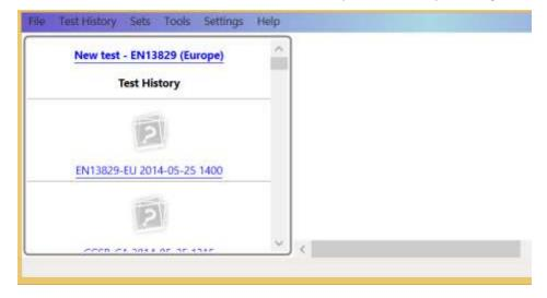
Make sure "New Test" on the history list is followed by "EN13829(Europe)". If not, go to "Settings" → "Change Standard used for new tests" and change the test standard to "EN13829(Europe)". You may need to restart the program if this change is not active immediately.
