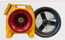
Both Retortec's Model 340x DuTester and The Energy Conservatory's Duct Blaster® are built to measure the airtightness of forced air heating, ventilating and air-conditioning ductwork.
