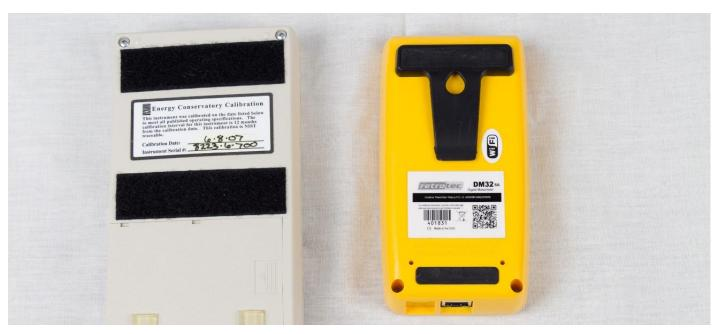
Velcro loops mount to a speed control plate that will clamp to a door.
