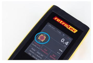
To start the test, tap the Power Button. Device and Range are shown as color image. Settings are saved.
