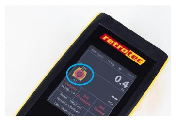
To start the test, tap the Power Button. Device and Range are shown as color image. Settings are saved.
