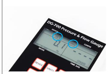
To start the test, press ON, then 10 clicks on 5 keys. Device and Range are shown as character codes. Settings are not saved.
