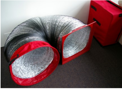
Flex-duct for ceiling neutralization
