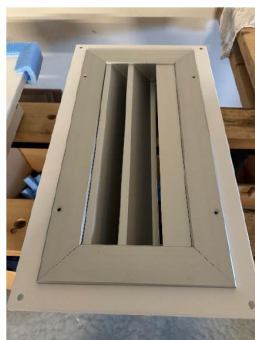
Fitting the louvre into the PRV opening Louvre seated in the PRV backside
