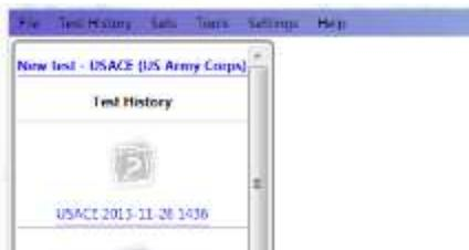
Make sure “New test” on the history list is followed by USACE. If not, go to “Settings” → “Change Standard used for new tests” and change the test standard to USACE. You may need to restart the program if this change is not active immediately.
