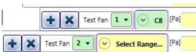
The fan number in the drop down next to "Test Fan" corresponds to the fan number in the list of fans you entered in the Equipment tab, see section 2.
