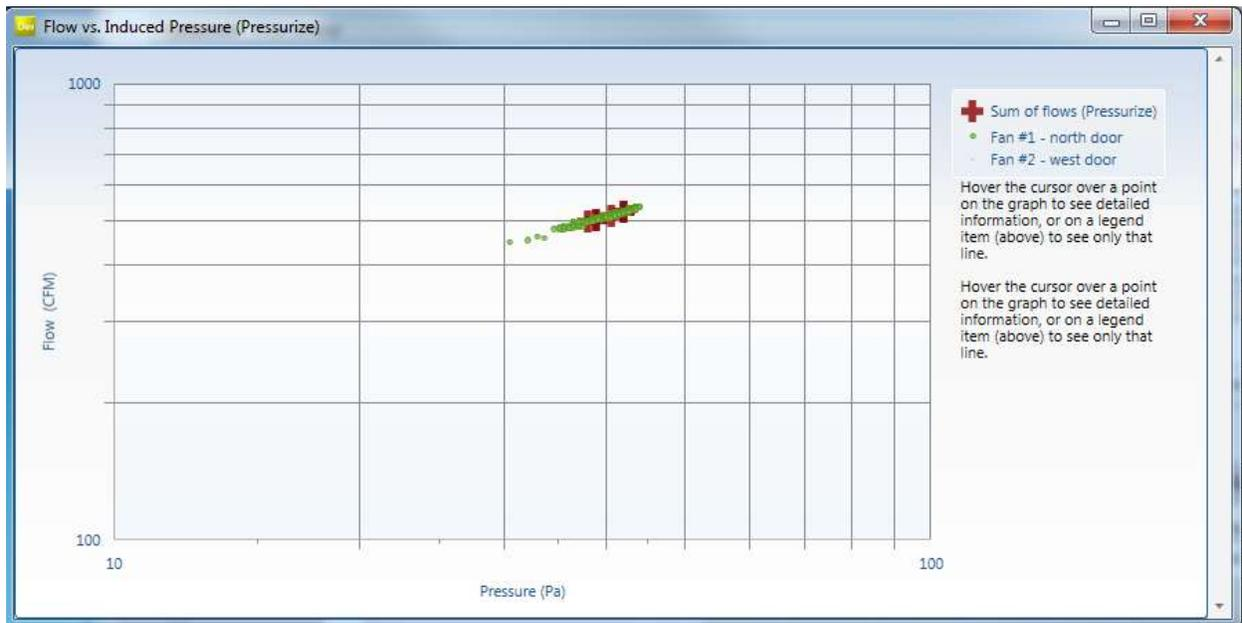
The number and location of the fan from which the readings are taken is shown on the graph legend, and moving the cursor over the points on the graph shows detail about each reading (pressure and flow at that point). The individual fan flow readings are shown, as is the sum of all flows in the case of the use of multiple fans.
