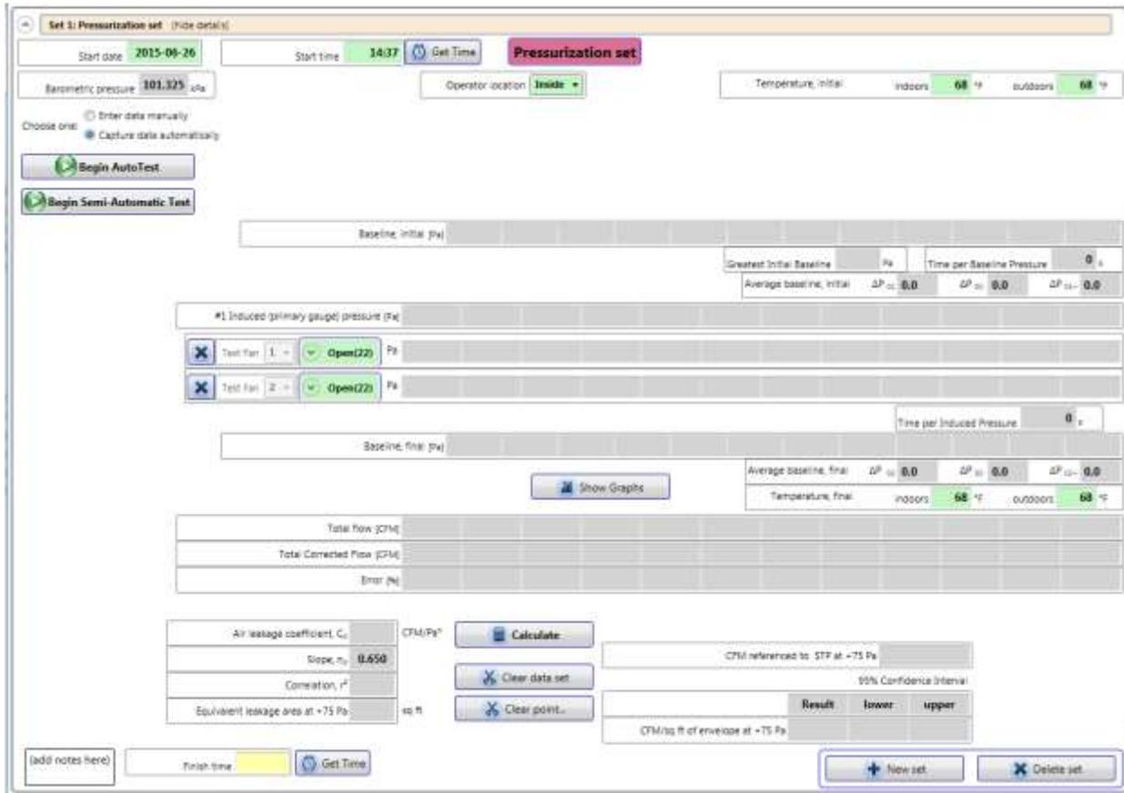
Data readings from each fan are specific to the range configuration installed on the fan when the pressure or flow is read from the gauge. A Fan Pressure Line must be included in the set for each fan/range combination used during the test (if ranges have to be changed during a test to reach the required induced pressure).
