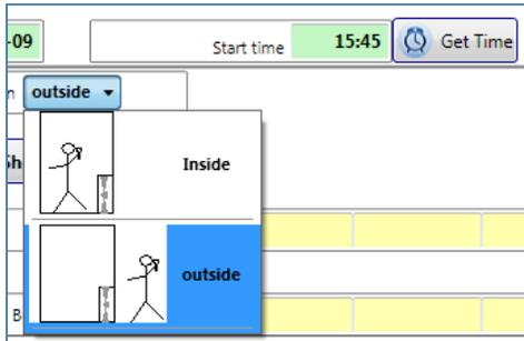
Select whether the operator is located inside or outside during the test (inside is typical). This is used in conjunction with the sign (positive or negative) from the Induced Pressure read from the gauge, to determine the test direction (Pressurization or Depressurization). The test direction will be displayed beside the Start time:
