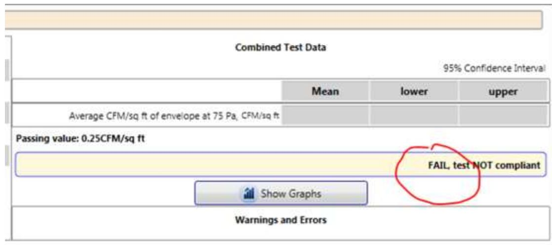
The “Passing value” for USACE Protocol is an average permeability for the building of less than 0.25 CFM/sq ft (based on results from a pressurize and depressurize data set).
