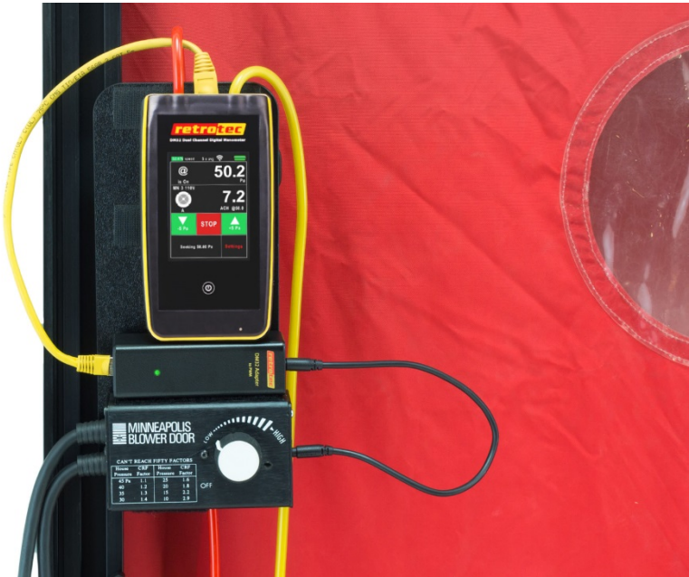
Figure 12: Control a TEC fan using the gauge and Fan Speed Control Adapter (part FN275, produced by Retrotec)
