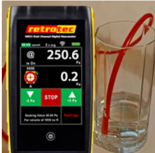
Figure 71: The gauge displaying a negative pressure (-250.6 Pa).
