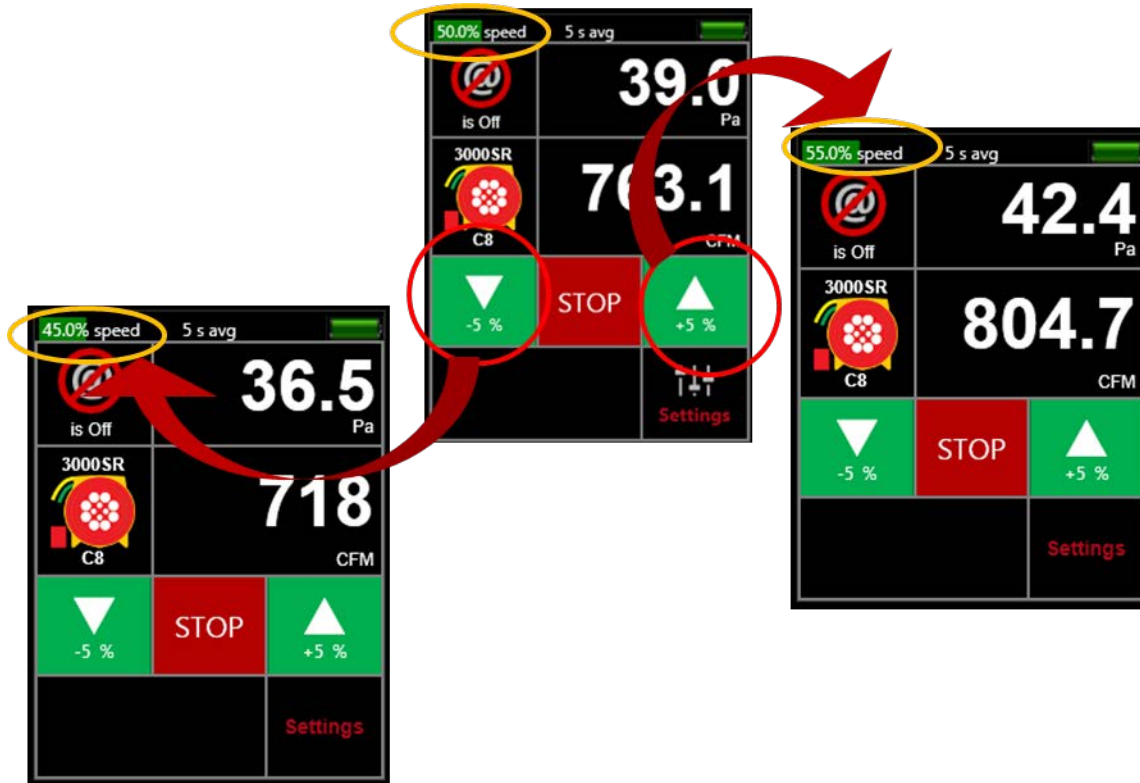
Figure 16: Adjust speed up or down 5% using [Jog] keys
