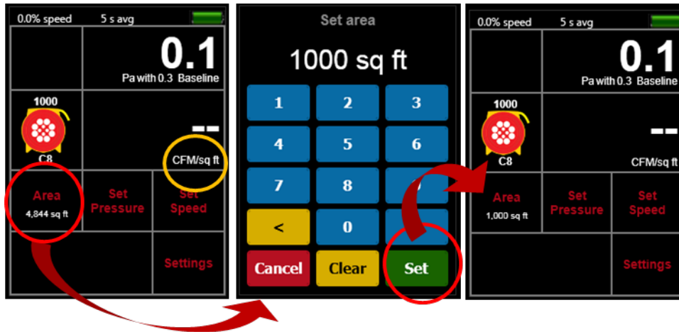
Figure 37: Set the [Area] needed for "per Area" type Results from the Home screen
