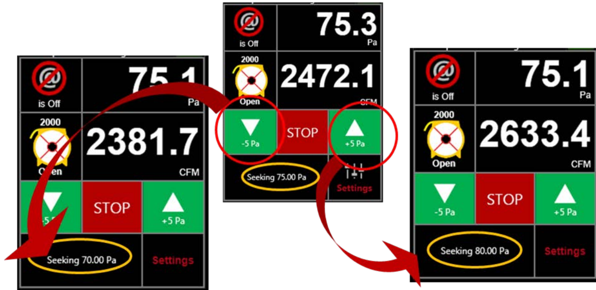
Figure 18: Adjust pressure up or down 5 Pa using [Jog] keys
