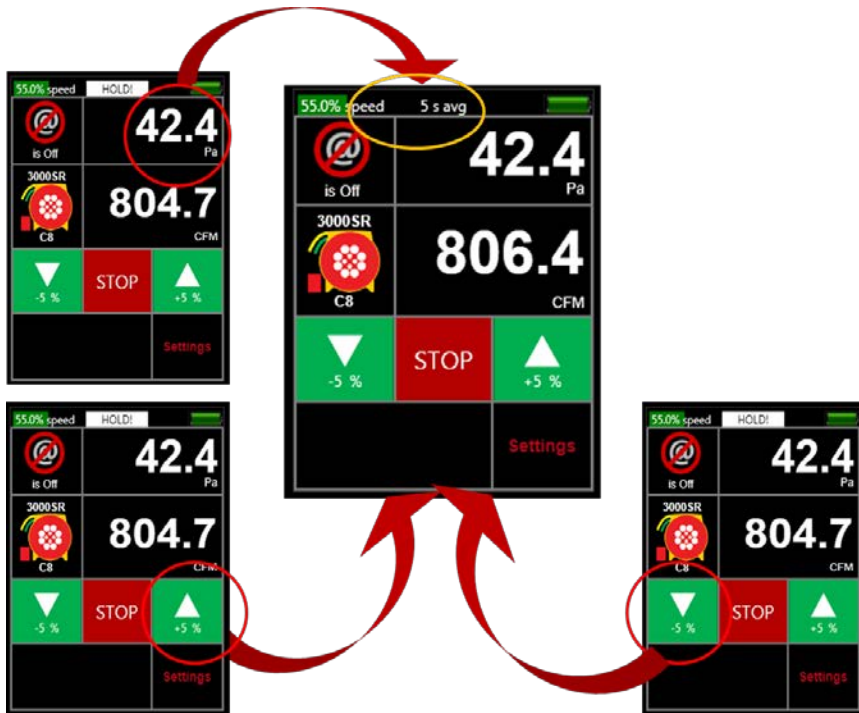
Figure 22: Remove "HOLD!" by tapping [Channel A] or a [Jog] key
