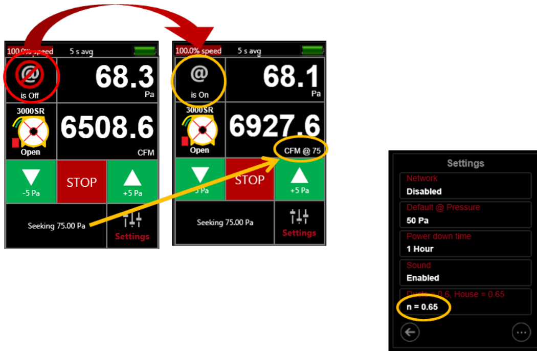
Figure 29: [ @ Pressure ] extrapolates to the target pressure when a pressure is set
