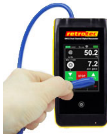
Figure 67: Errors in pressure reading from a pinched tube.
