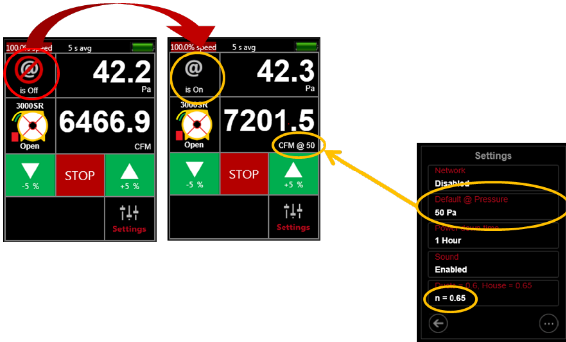
Figure 31: [@ Pressure] extrapolates to “Default @ Pressure” when a speed is set
