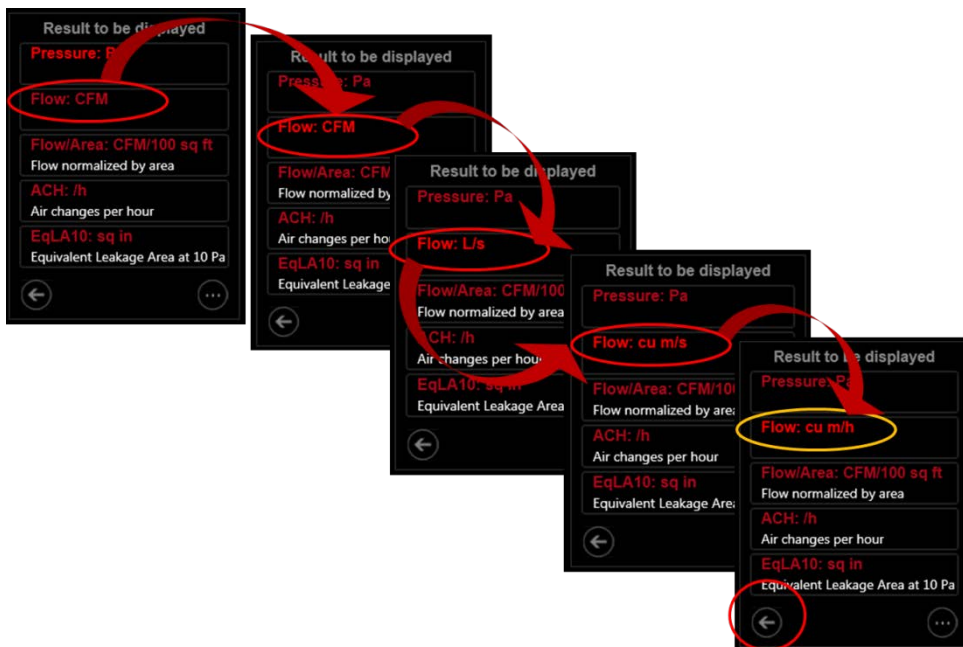
Figure 25: Change Flow result units from “CFM” to “cu m/h”
